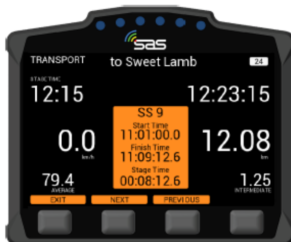
SCREEN 14. Times of completed stages
